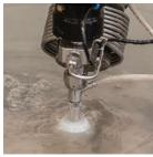
Automatic water Raise/Lower at the push of a button for Submerged Cutting; our tanks include air-tight welds of an air chamber which uses regular shop air pressure.
