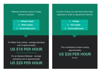
If we are simply looking at operating costs then both Laser and Waterjet cutting have similar costs. However, a typical waterjet machine will cost about half what a CNC Laser will cost for a similar size and quality. Therefore, when the machine cost is also amortized into the total operating cost, the waterjet will end up being considerably less than the CNC laser.
