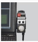
The MPG allows to manually wind forward or backward through a cutting path. This enables the operator to find the exact point along a cutting path from which to re-start cutting after a stoppage, or to accurately locate a pre-cut part.
