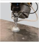
Automatic water Raise/Lower at the push of a button for Submerged Cutting; our tanks include air-tight welds of an air chamber which uses regular shop air pressure.
