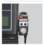
The MPG allows to manually enables the operator to find the exact point along a cutting path from which to re-start cutting after a stoppage, or to simply locate a pre-cut part.
