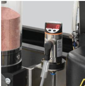
Tech-Sense Monitoring System enables true unattended operations. Should the cutting be disrupted the machine will pause the program and send a text message to your cell phone (SMS Notification option must be fitted.)
