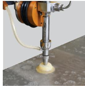
Automatic water Raise/Lower at the push of a button for quieter, cleaner and safer submerged cutting; our tanks include air-tight welds of an air chamber which uses regular shop air pressure.
