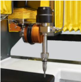
Should the cutting head inadvertently crash into a clamp/fixture, hit the edge of a work piece or an upturned part, the Break Away Head will detect the crash and automatically stop the machine.
