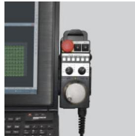
The MPG allows to manually wind forward or backward through a cutting path. This enables the operator to find the exact point along a cutting path from which to re-start cutting after a stoppage, or to simply locate a pre-cut part.
